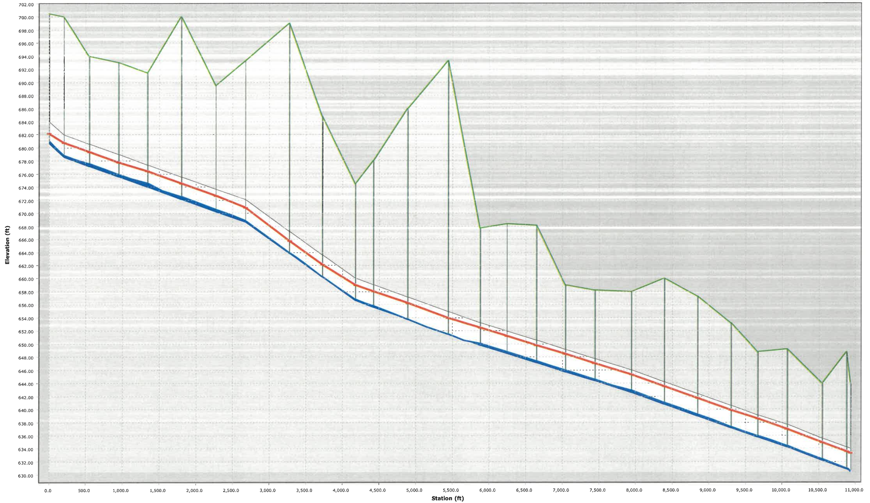
Future Design Max Flow Conditions (August 30 Event) without Sluice Gate and Pumping Station Route B 42-Inch Pipe
